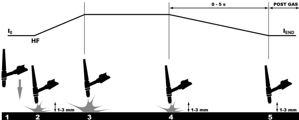
Picture 1 - welding process at TIG HF
