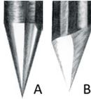
**Picture 5A** - fine and even grinding of the electrode in the longitudinal direction - lifetime up to 17 hours
